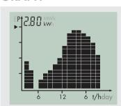
The inverter energy is shown as a diagram on the display. The daily graph is displayed by default. The right-hand flashing bar of the diagram represents the current hour. If the inverter does not feed any power to the grid over a longer period of time (e.g. in darkness or if the PV modules are covered with snow), a gap is inserted into the chart. The column for the current hour is updated automatically every five seconds.
